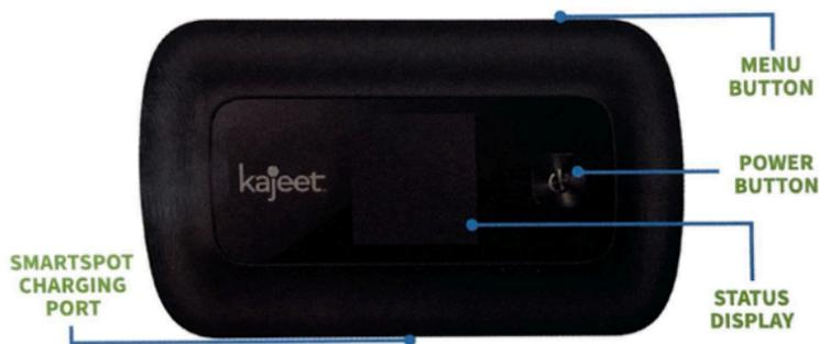
**POWER BUTTON:** Powers the Kajeet SmartSpot on and off and wakes the device from sleep. This button is also used as the 'OK' button when browsing through the menu.
